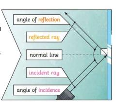
The angle of incidence is the angle between the normal line and the incident ray of light.
